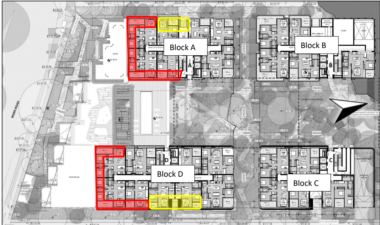
Figure 5-1 Markup for Traffic Intrusion Requirements for Glazing
